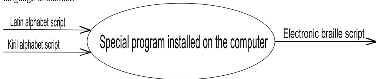
Picture 1. The principle of operation of a converter that translates records from different alphabets to the Braille
